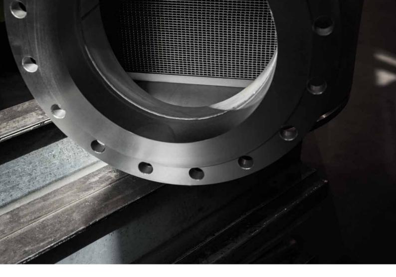
Shell side view of new 5SH plate pack. Instead of the round shape of the original plate, the new plates use the shape of an athletics field.
